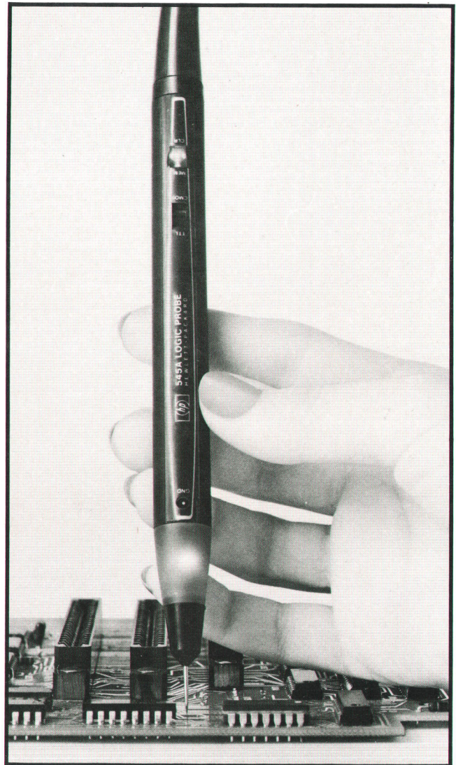
Fig. 1. Model 545A Logic Probe indicates logic levels and pulse activity at individual digital circuit nodes.
