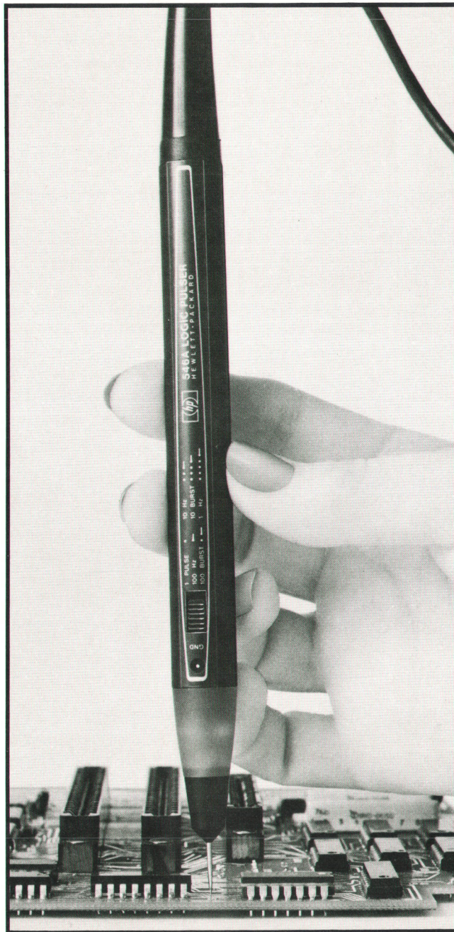
Fig. 1. Model 546A Logic Pulser provides single pulses, pulse bursts, and pulse trains that automatically drive a digital circuit node to its opposite state.
