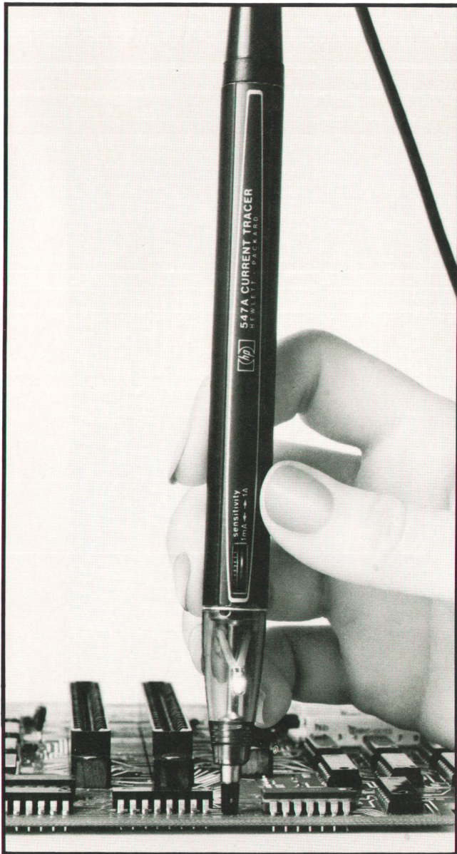
Fig. 1. The lamp near the tip of the new Model 547A Current Tracer varies in brightness according to the relative magnitude of the current steps occurring near its tip. By observing how the lamp's brightness changes as the tracer is moved along the conductors the user can follow the flow of current.
